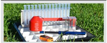
Included as standard to assist with the correct set-up and testing of the rate, flow and distribution pattern of products. The kit includes 13 test trays with dividing inserts, test tubes, bulk density meter, hardness tester, granular sieve, and a windometer.
