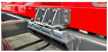
The AS2000 loadcells are standard on all models. Four point load cells ensure spreader acuracy at all times with all products. The load cells can callobrate the rate on the go and adjust the CAL factor for products of variaing bulk density.
