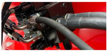
The AS2000 hydraulic valve assembly is compatible with tractors using load sensing hydraulics.
