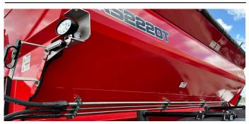
The AS2000 has a stainless steel bin, along the front rear and bottom third, providing longevity.
